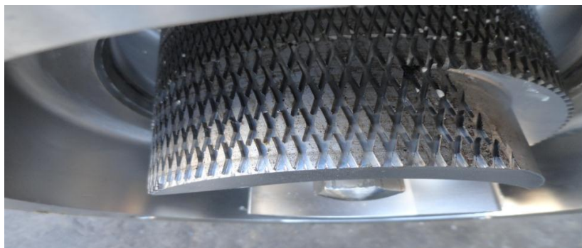
Figure 3: The grinding rotor-stator system
