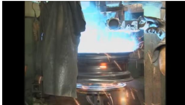
Figure 11. Mig-Mag Welding among rim and the disc, source: Rodabrás
