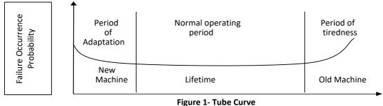
For Slack et al. (2001), this figure represents a typical curve of an equipment life; it is comprised three different stages in it:
