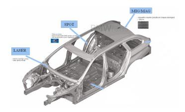
Figure 2. Types of weld done in BIW
