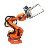
Fig. A.8. MIG/MAG welding robot
