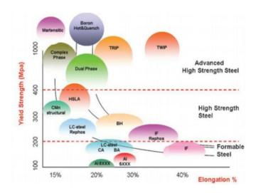
Fig A.4. Main steels used in the BIW body
