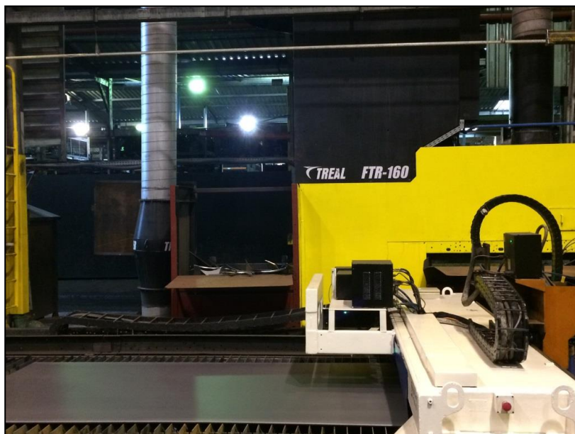
Picture 9 PLASMA CUTTING – ASPIRATION SYSTEM
